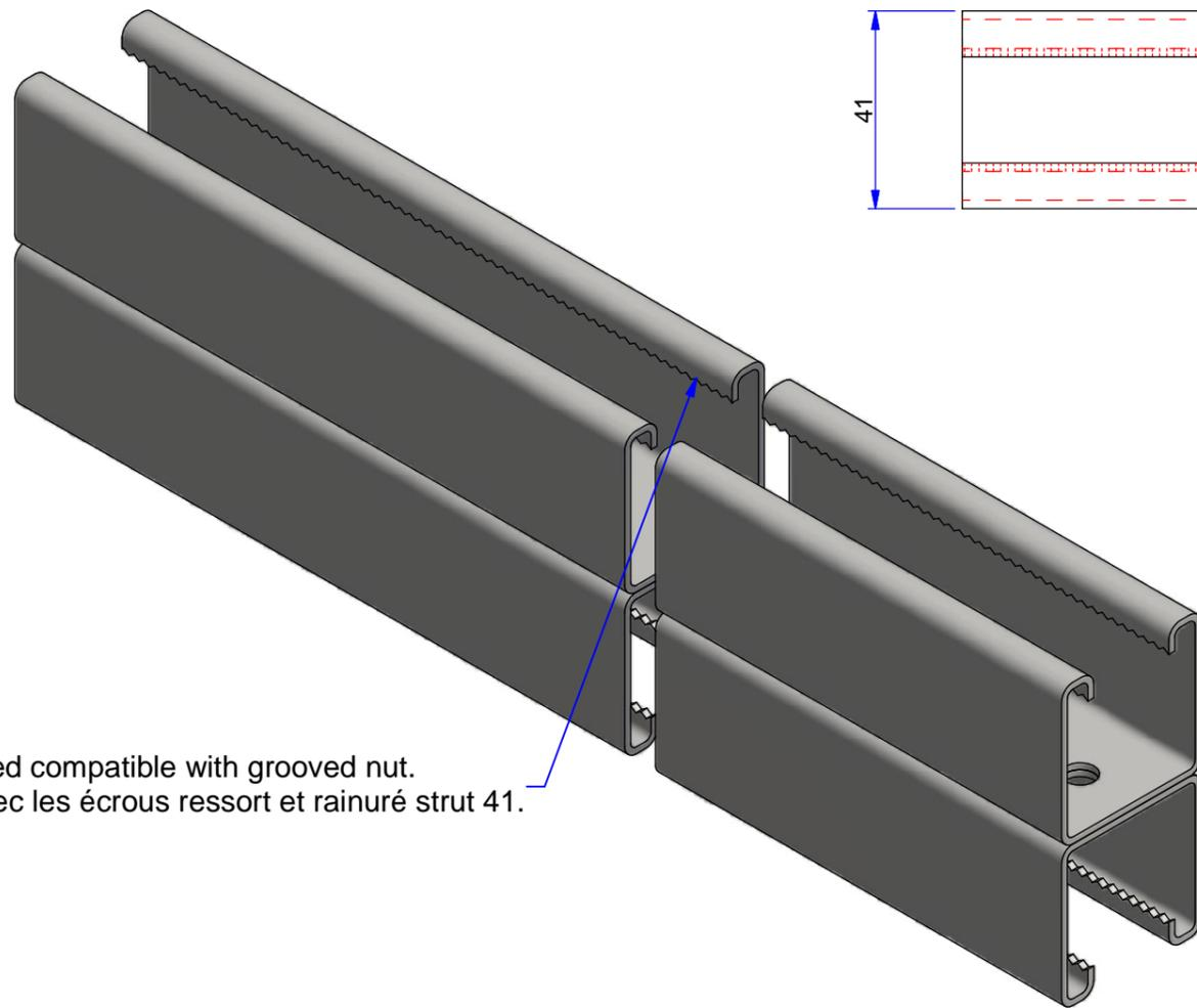
Rail notched compatible with grooved nut.
